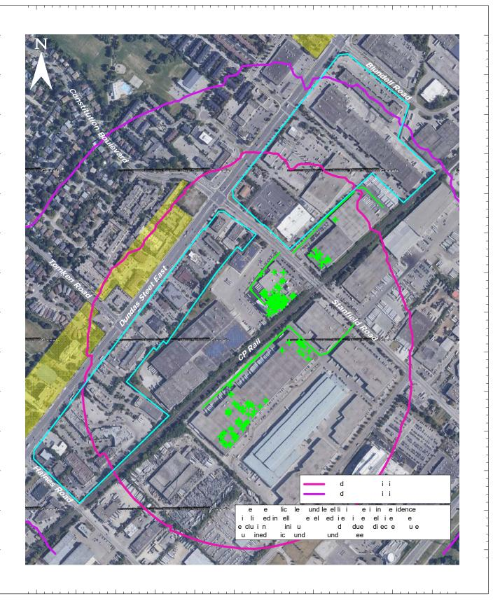
Figure 3: Sound Level Contours, Leq [dBA], at Elevation Representative of 15th Storey
