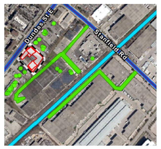
3. The actual situation, recognizing all of the noise sources utilized by HGC Engineering is significantly different, as can be seen in the number and location of the actual noise sources shown as green crosses and lines:
