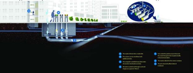
At Wembley Park, waste is transported underground via three separate chutes to a local collection center for pick-up and removal, reducing contamination of waste streams as well as truck traffic. (Credit: Envac)
